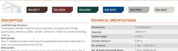
Walls in sandwich panels consisting of two galvanised sheet layers filled with an inner core of polyurethane foam (PUR).
