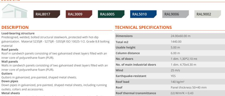
Galvanized, pre-painted, shaped metal sheets for ridges, corner joints, flashings and eaves and any other necessary element.
